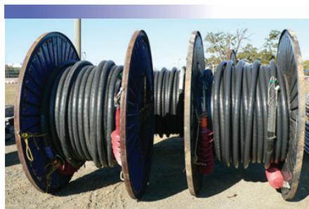
*Temporary cables are wound onto large reels and moved from project to project.*
