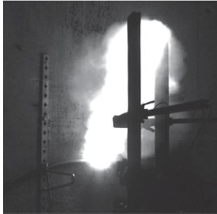
Arc flash resulting from a cable fault.
