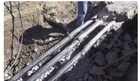
Buckling of three 66 kV XLPE cables in 2011 earthquake in Christchurch, New Zealand (courtesy Orion Electric).
