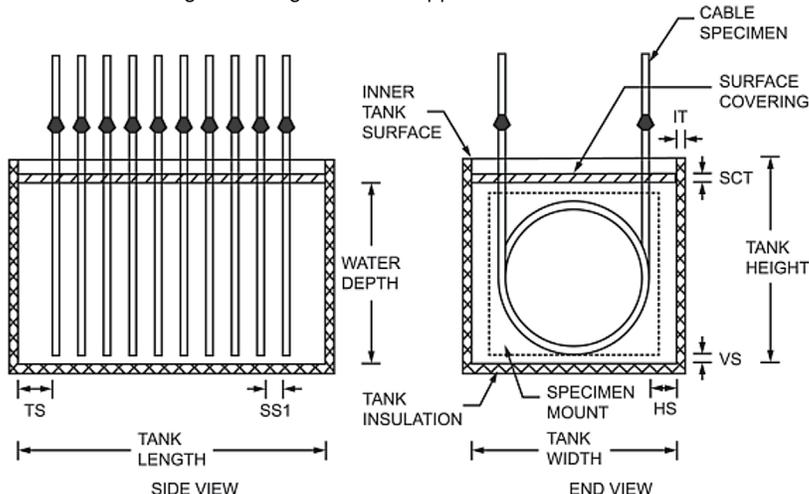
Typical setup for ACLT from IEEE 1407
