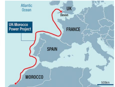
Figure 1: Possible route for 4 x 3800 km HVDC submarine cables from Morocco to UK (credit: www.xlinks.co/morocco-uk-power-project)
