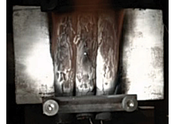
Figure 1. Image of three parallel cable samples being exposed to focused solar thermal radiation
